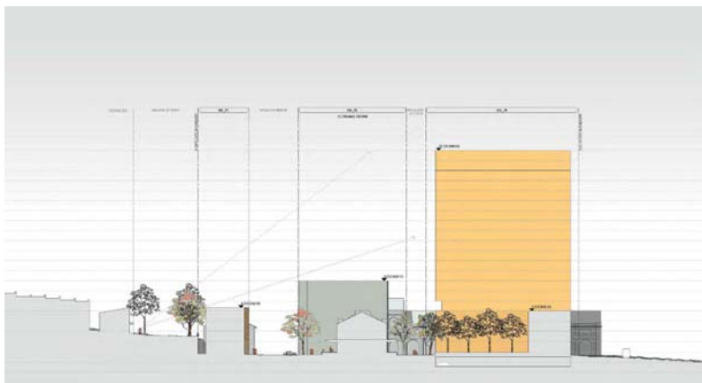
North-south cross section through the site showing proposed development from the north side of Wilson Street. Analysis shows that buildings will be obscured by existing mature street trees
